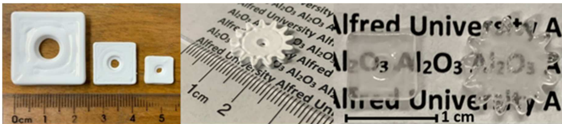
Fig. 1. Photographs of 3D printed alumina ceramics of varying shapes and sizes
